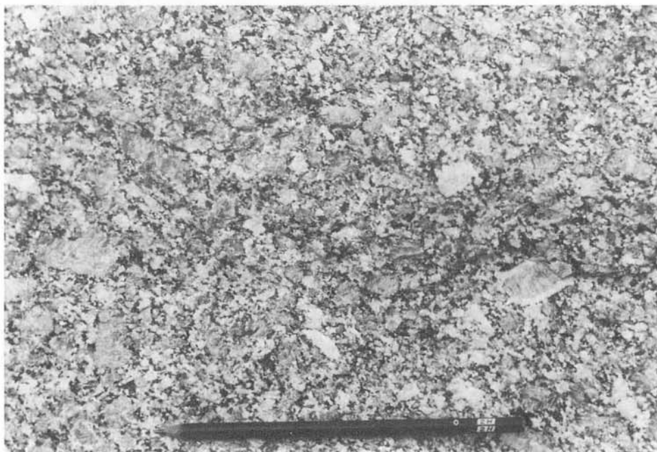
Plate 7. Noring Granite ( Belimbing facies ). Pink potash feldspar megacrysts, occasionally rimmed by plagioclase, in a coarse, unfoliated groundmass of quartz-plagioclase-biotite-hornblende. (East-West Highway; Grid Ref QU 135238).
