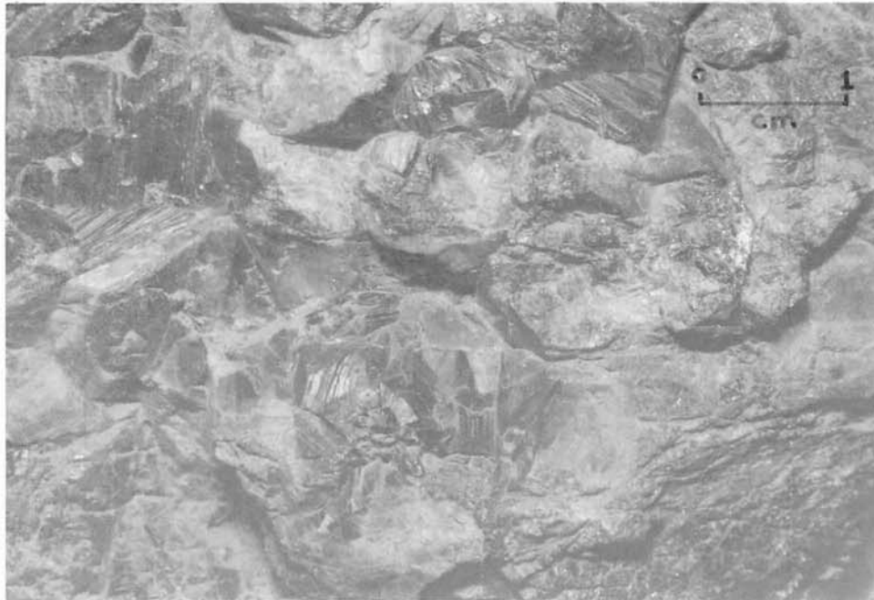
Plate 1b. Mottled nature of the same lode which is characteristic of many hydrothermal lodes. Colours range from pale yellow, yellow brown to dark brown and black. Colour of pegmatitic cassiterite is usually not so variegated and is quite typically black. Loc: From a mine in Suratani Province, Thailand.
