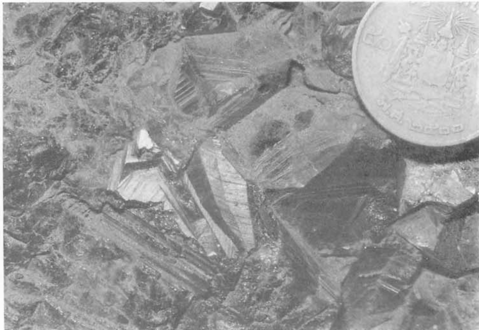
Plate 1a. Close up view of cassiterite twinnings and zoning of a pure cassiterite lode. Cyclic twins and zoning are present. This cassiterite lode is hydrothermal in origin. Size of coin is about 2 cm. Loc: From a mine in Suratani Province, Thailand.
