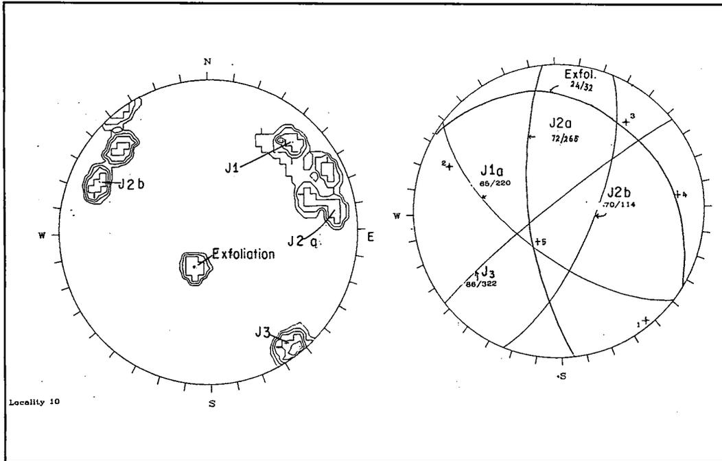
Figure 3: Pole concentration and joint plane plots at locality 10 indicating dip and dip direction of each joint set.
