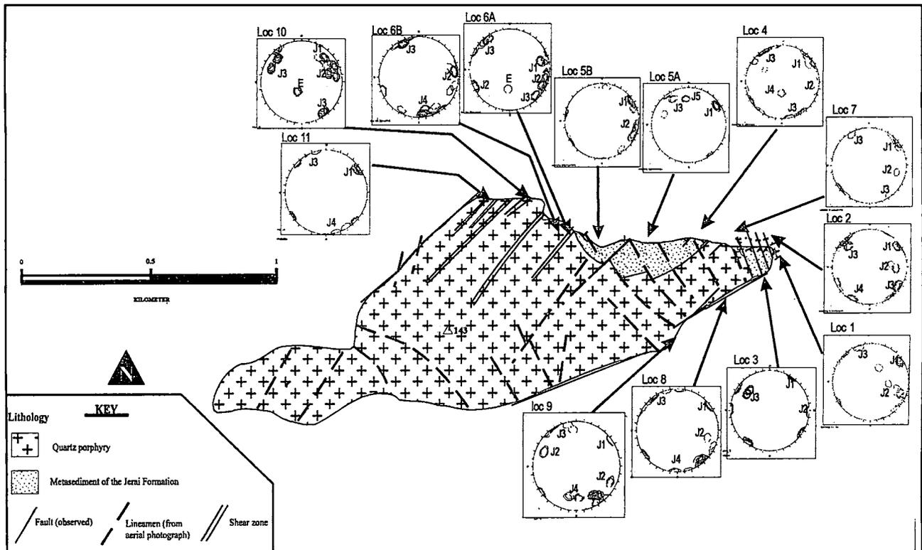
Figure 4: Geological map and joint orientation pole plots at various localities.
