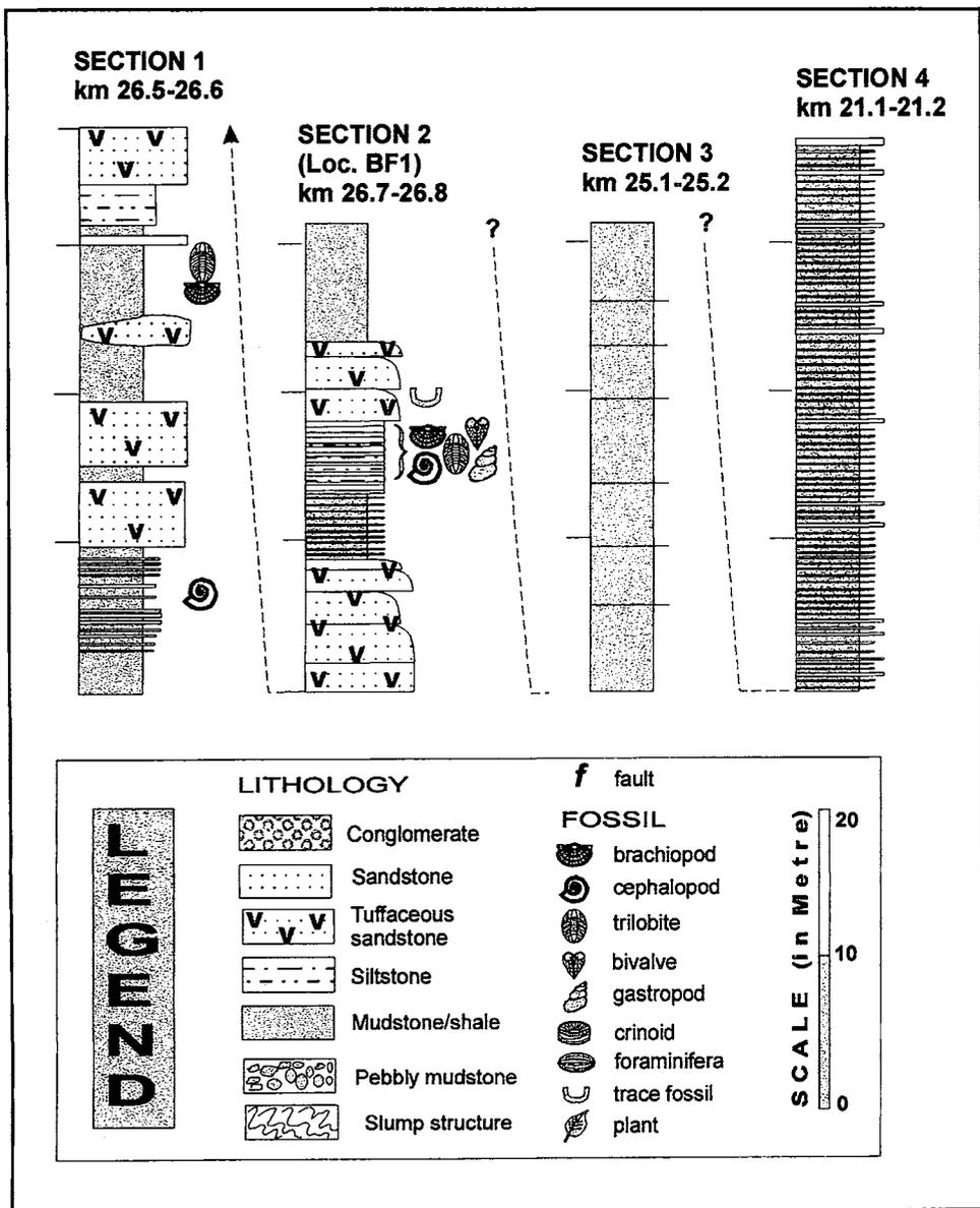
Figure 2: Sedimentological logs for major sections of the lower part of the Bera Formation.
