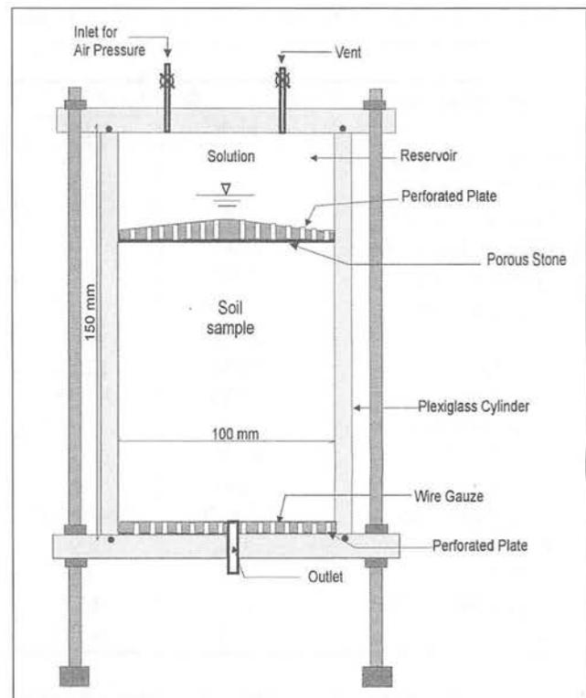
Figure 2: The laboratory leaching cell (modified from Tan, 1993 and Reid and Brookes, 1999).
