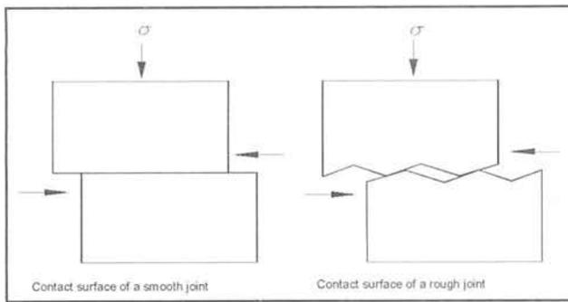
Figure 3: Gross contact area of joint surface.
