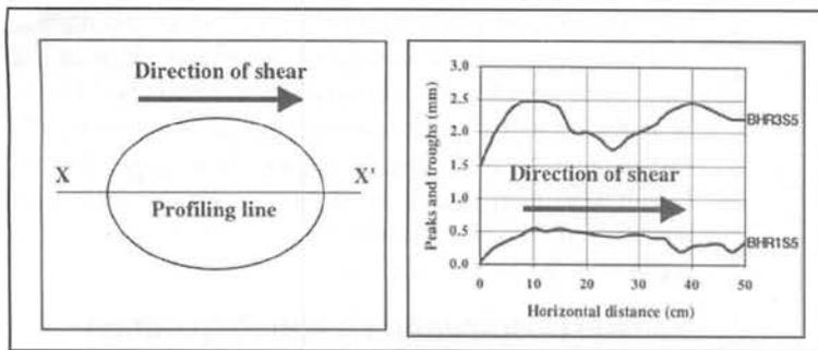
Figure 6: Typical joint roughness profiled along the direction of shear.
