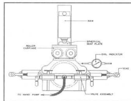
Figure 5: Shear box and loading rams.
