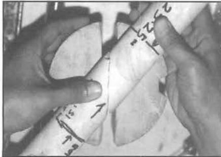
Figure 7: Jointed core sample.
