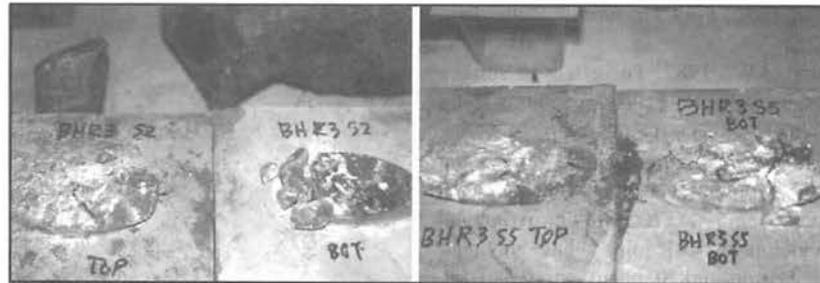
Figure 11: Crushing of joint asperities.
