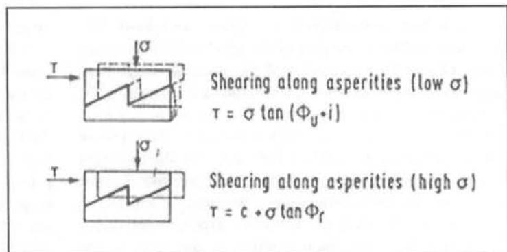
Figure 2: The mechanics of failure of rough joint
