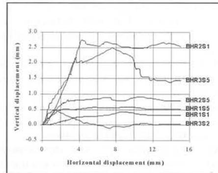
Figure 10: Vertical displacement vs. shear displacement.
