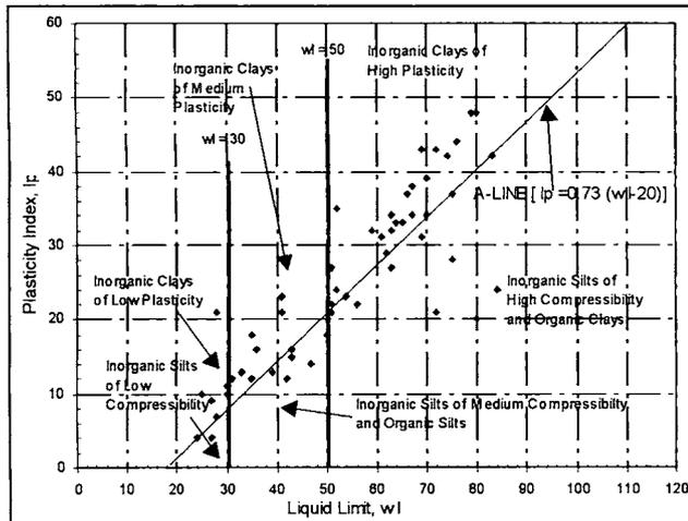
Figure 10: Correlation between the Atterberg limits using the plasticity chart (after Casagrande, 1932 in Terzaghi & Peck, 1995).
