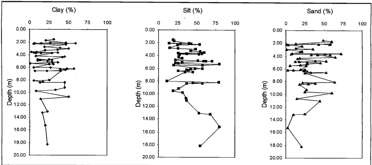
Figure 4: Plots of clay, silt and sand contents with depth.
