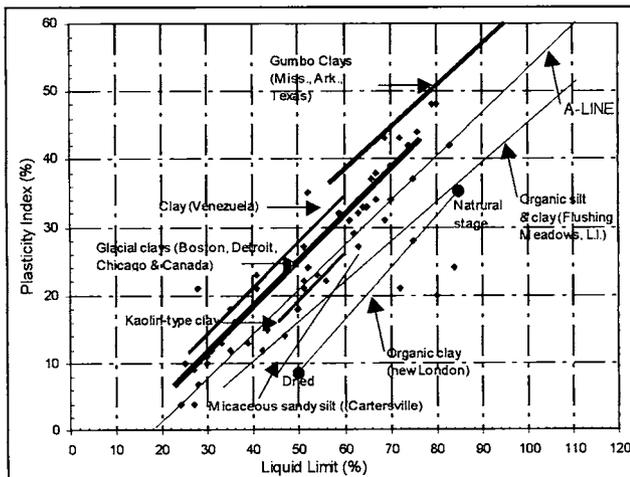
Figure 11: Relationship between Liquid Limit and Plasticity Index for typical soils (after Casagrande, 1932 in Terzaghi & Peck, 1995).
