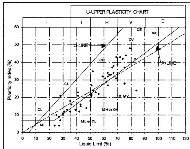
Figure 8: Modified plasticity chart for use with Unified Soil Classification system. Soil represented by points within shaded area are considered borderline and are given dual symbols (after USBR, 1974). Note: L:low; I:intermediate; H:high; V:very high; E:extremely high; M:silt; and C:clay.
