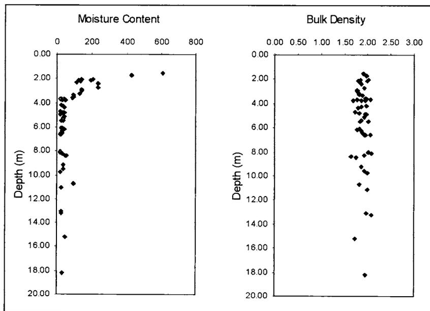
Figure 3: Plots of moisture content and bulk density with depth (m).
