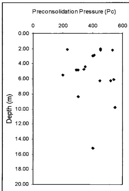
Figure 7: Plot of preconsolidation pressure (Pc) with depth.
