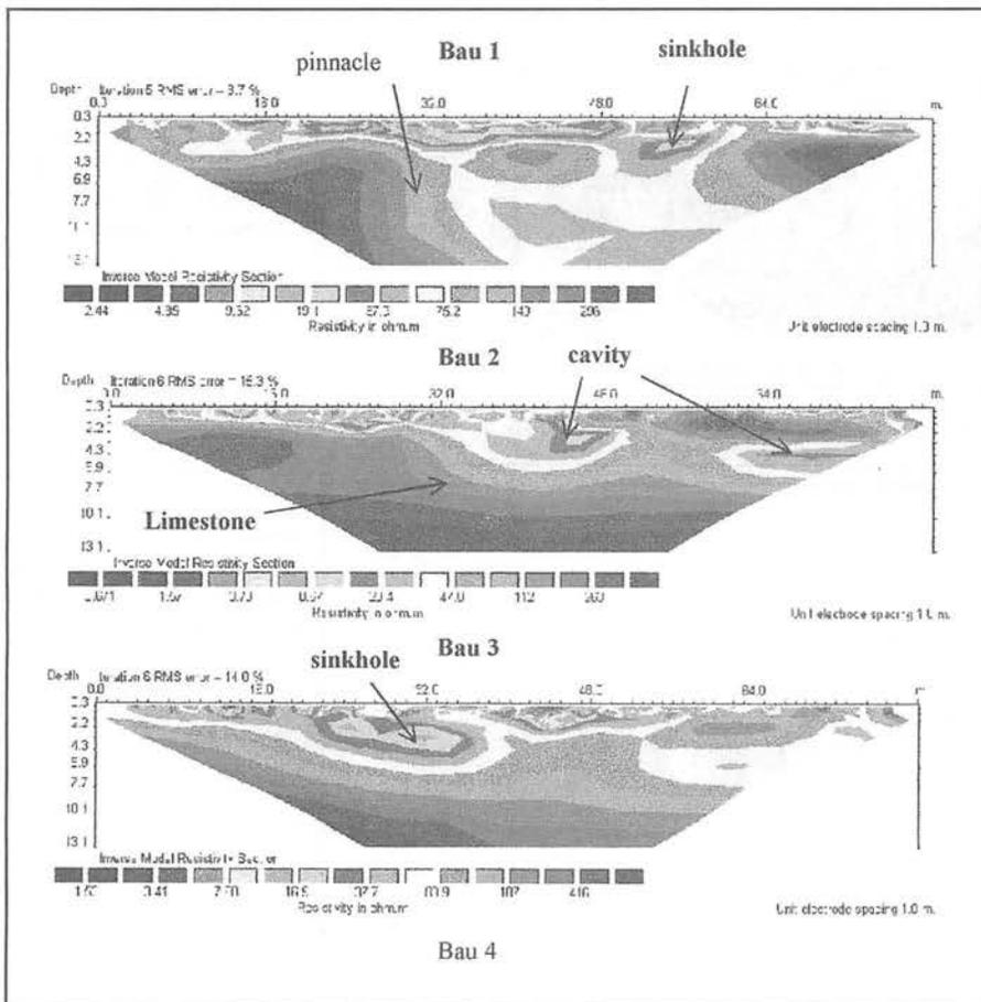
Figure 2: Resistivity inverse models showing locations of sinkhole and cavity.
