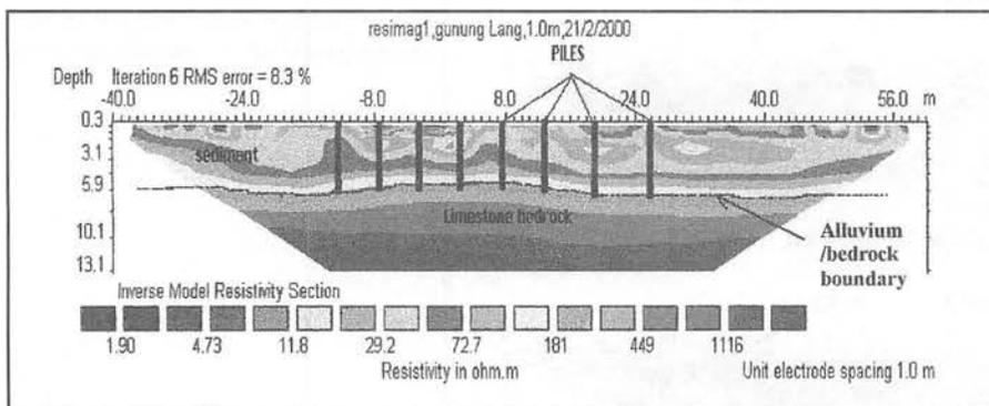
Figure 3: Resistivity inverse model showing location of piles resting on a regular and almost flat subsurface topography of limestone bedrock.
