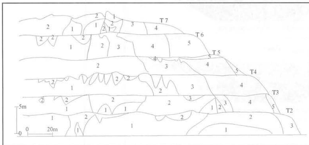
Figure 4: Weathering profile index of quartz mica schist slope cut at km 67, Grik-Jeli highway, Perak.
