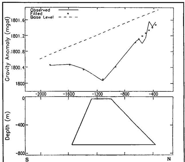
Figure 5: Gravity model of anomaly B.
