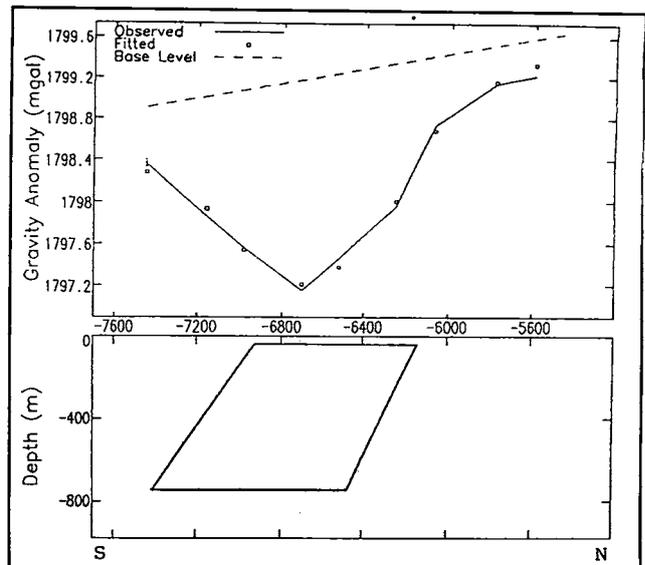
Figure 4: Gravity model of anomaly A.
