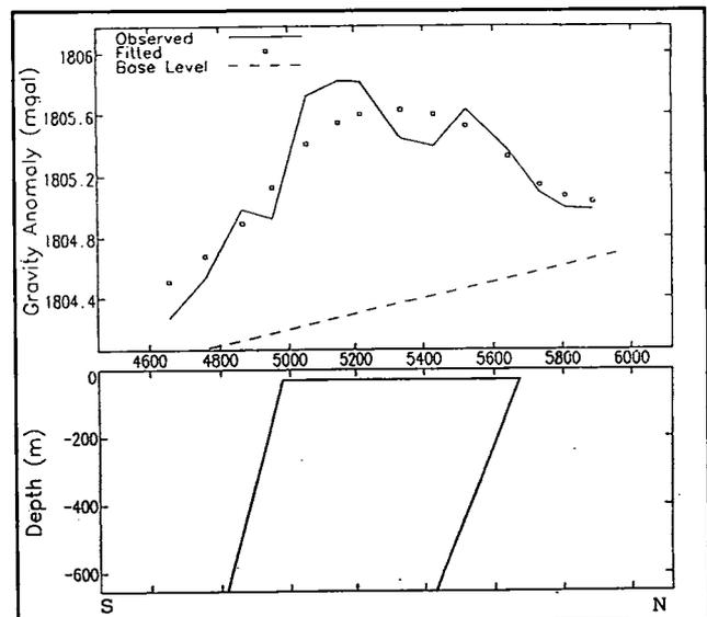
Figure 6: Gravity model of anomaly C.
