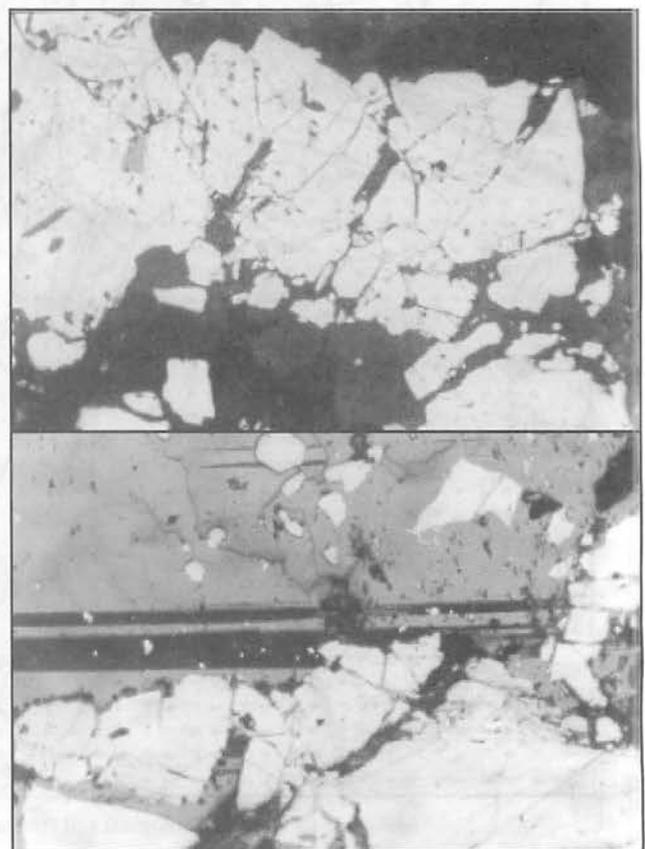
Figure 3. Photomicrographs showing cataclastic texture in pyrite and chalcopyrite filling the fractures in pyrite (top) and gold and chalcopyrite filling in pyrite fractures (bottom).
