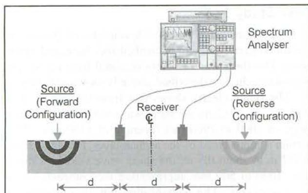
Figure 2. Basic configuration of equipment for SASW measurements.
