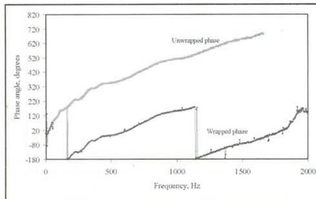
Figure 5. A typical phase plot of the cross power spectrum from SASW measurement on asphalt pavement for a 100 cm receiver spacing.
