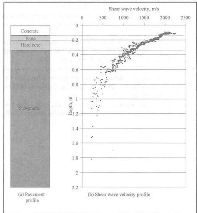
Figure 8. Comparison between the actual inverted shear wave velocity profiles from SASW measurements on a rigid pavement site.
