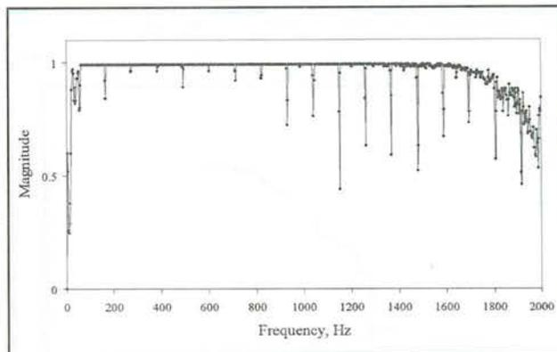
Figure 4. Coherence function of spectral analysis measurement on asphalt pavement for a 100 cm receiver spacing.
