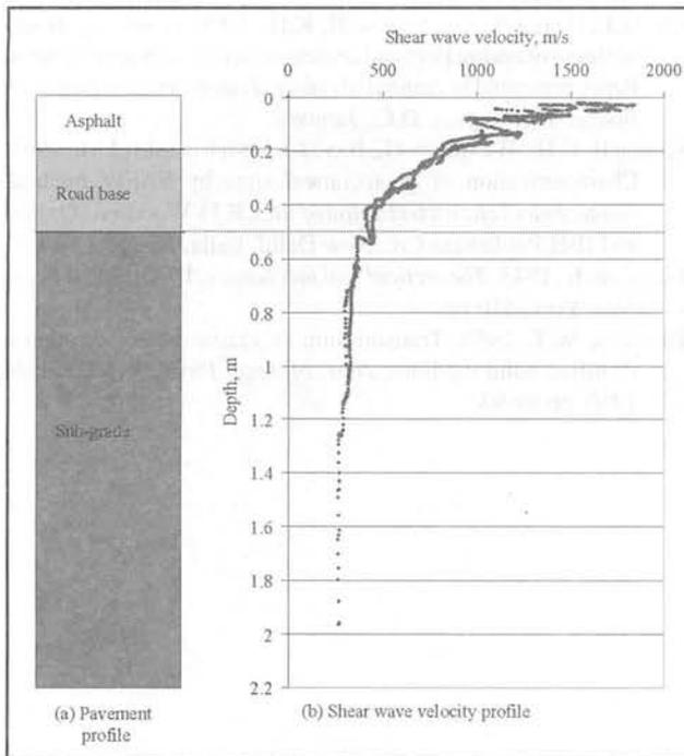
Figure 7. Comparison between the actual inverted shear wave velocity profiles from SASW measurements on a flexible pavement site.
