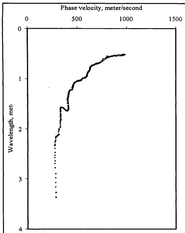
Figure 6. Dispersion curve constructed from record shown in Figure 5.
