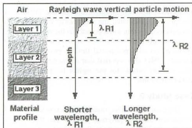
Figure 3. Variation of vertical particle motion for Rayleigh waves with different wavelengths.
