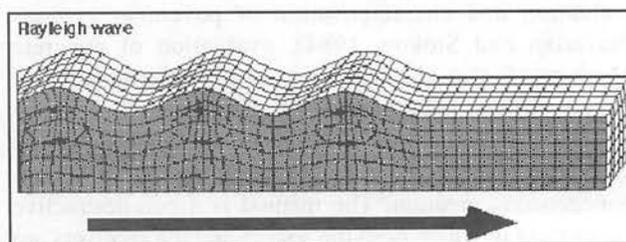
Figure 1. Elastic deformations and ground particle motion associated with the propagation of Rayleigh waves. Modified from Bolt (1978).
