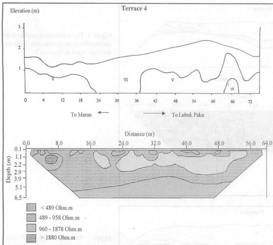
Figure 3. The weathering profile (top) and resistivity inverse section (bottom) for rock mass at Terrace 4
