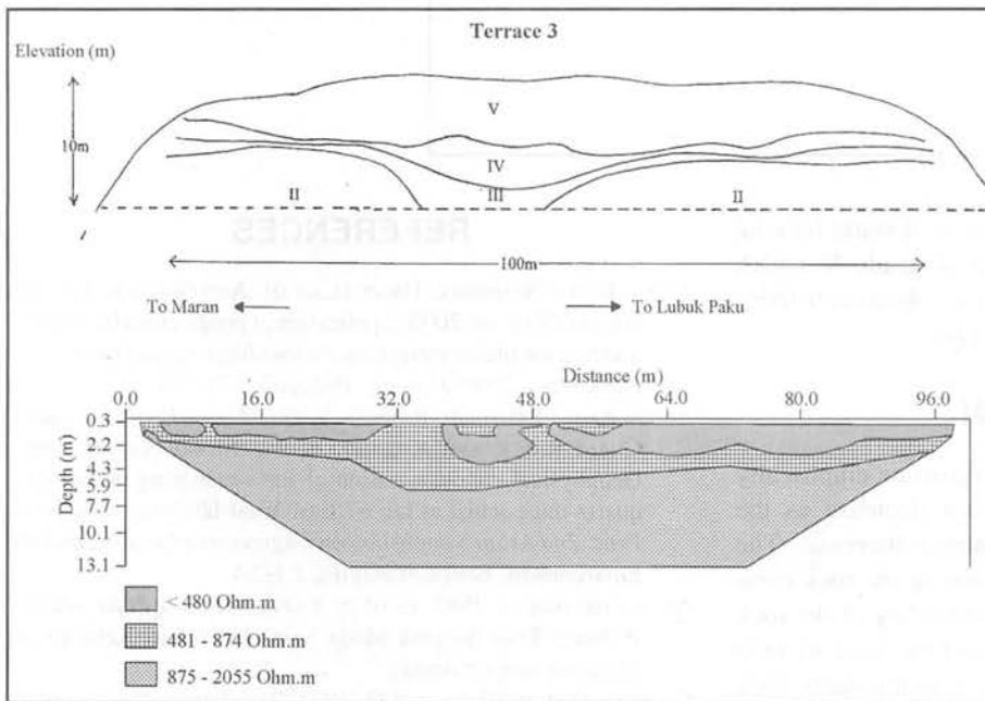
Figure 2. The weathering profile (top) and resistivity inverse section (bottom) for rock mass at Terrace 3
