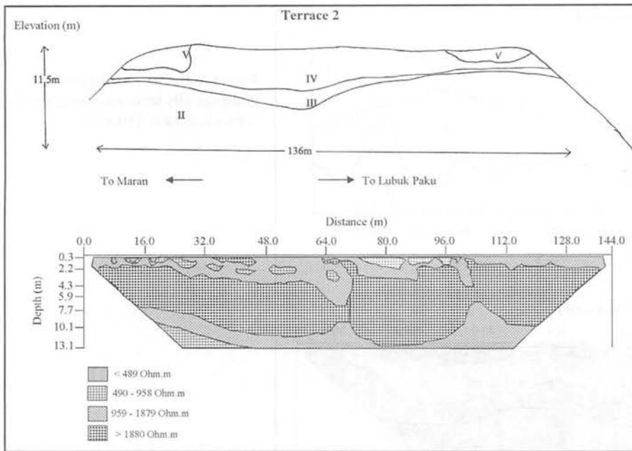
Figure 1. The weathering profile (top) and resistivity inverse section (bottom) for rock mass at Terrace 2
