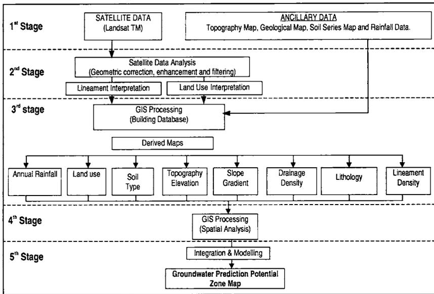
Figure 2. Methodology flowchart for groundwater potential zone mapping.
