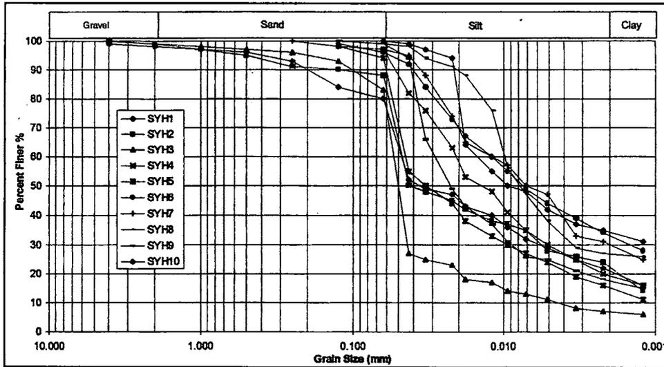
Figure 1. Grain size distribution curves.
