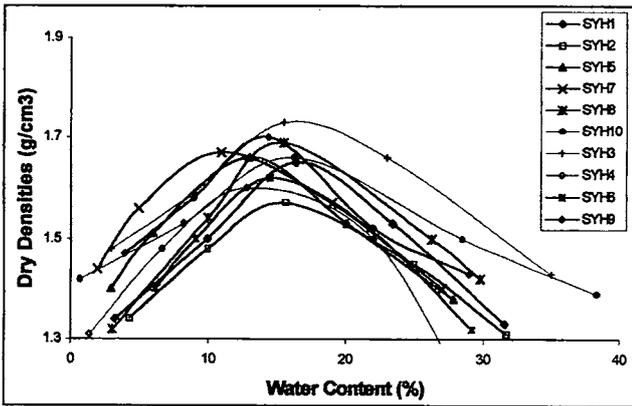
Figure 3. Compaction characteristics.
