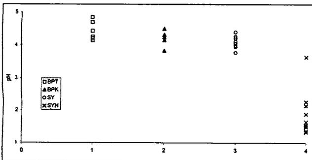
Figure 4. pH of pore fluids. SYH is residual soil from carbonaceous or black shale. BPT and BPK are residual soils from sandstones, while SY is residual soil from non-carbonaceous shale.
