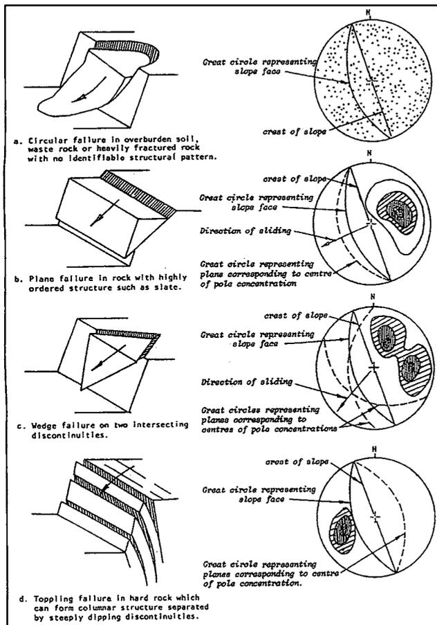
Figure 4. Main types of slope failure and stereoplots of structural conditions likely to give rise to these failures (Hoek and Bray, 1981).
