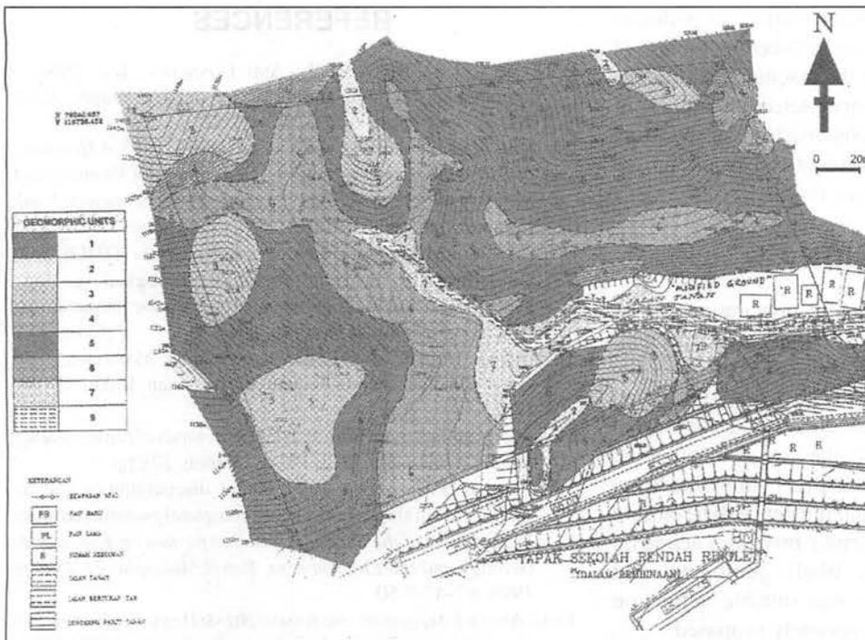
Figure 5. Map showing the zonation of the existing slopes/landforms based on the geomorphic units.
