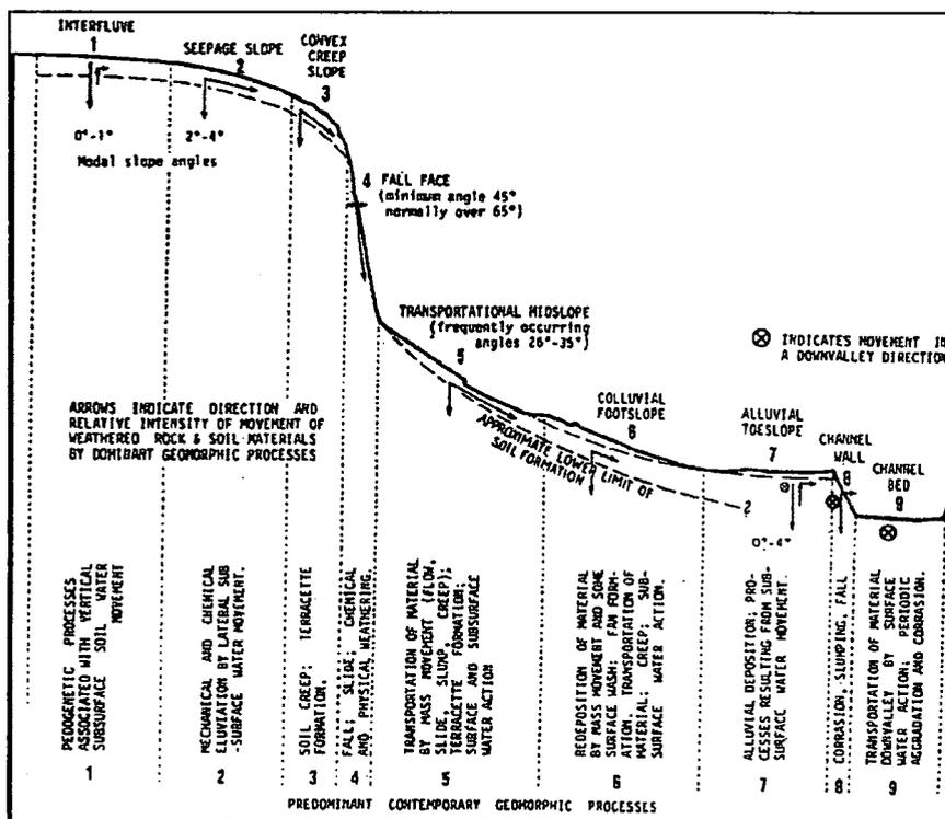
Figure 3. Classification of slope units and the associated predominant geomorphic processes (after Dalrymple *et al.*, 1968).
