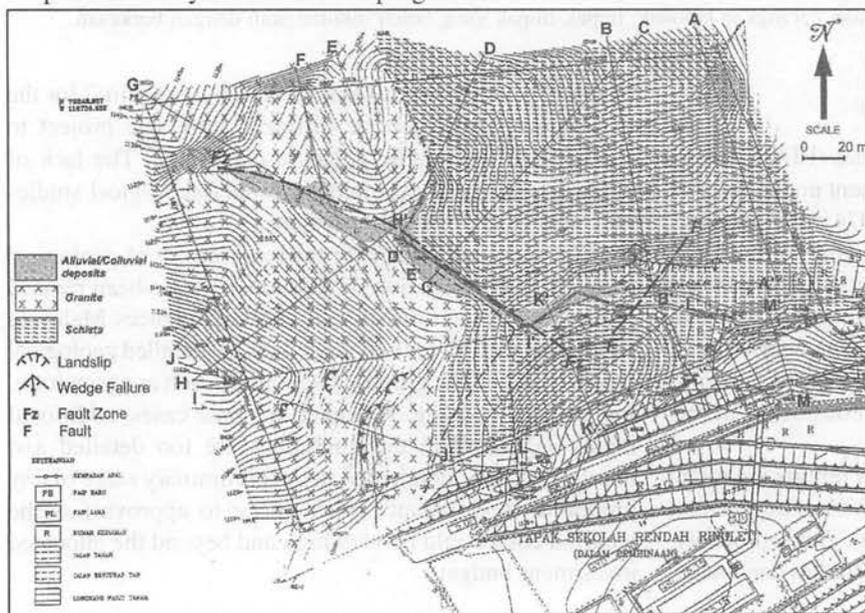
Figure 2. General geological map of the project site. Cross sections along A-A' to M-M' are shown in Figure 4.
