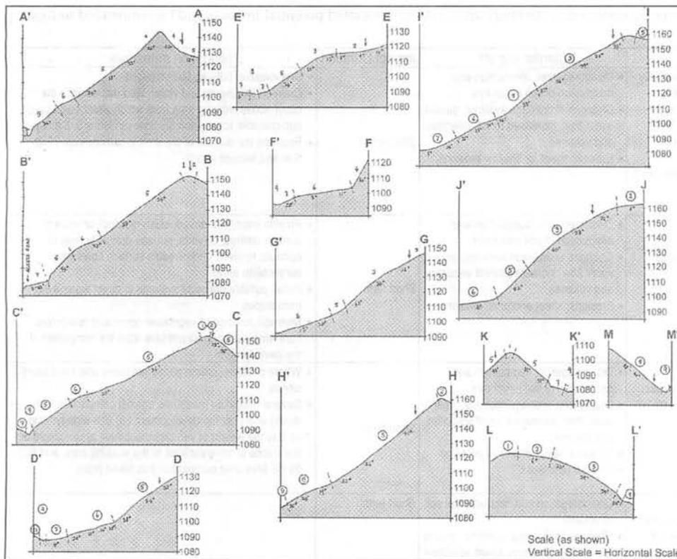
Figure 4. Cross sections showing the profile and classification of the geomorphic units.
